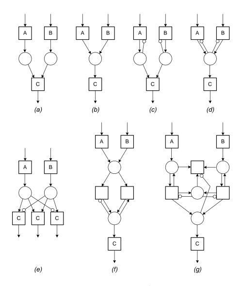
Fig. 1. Seven frequently used ways to join two flows (expressed in terms of Petri nets with inhibitor arcs [21]).
