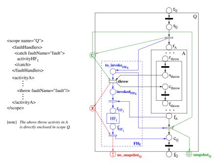
Fig. 14. Handling a process-defined fault generated by the throw activity.
