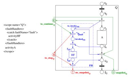
Fig. 13. A fault handler (general mapping).
