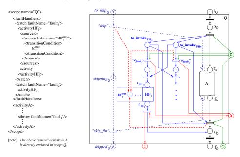
Fig. 18. Dead path elimination for a control link leaving from a fault handler.
