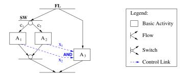
Fig. 1. An example of an unreachable activity (where control links are denoted by dashed lines).
