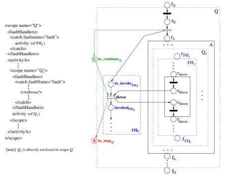
Fig. 16. Handling a fault thrown from within a fault handler.
