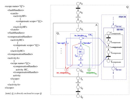
Fig. 19. Handling compensation invoked by the compensate activity.
