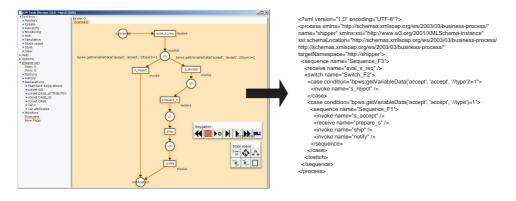
**Fig. 4.** The Petri net describing the service offered by the shipper is mapped onto BPEL code using WorkflowNet2BPEL4WS, a tool to automatically translate colored Petri nets into BPEL template code.
