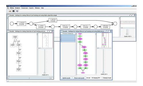
Fig. 12. The output of three process discovery algorithms supported by ProM when analyzing the event log shown in Table 1.
