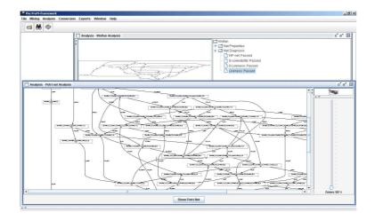
Fig. 2. Two analysis plug-in of ProM indicate that the Petri net shown in Figure 1 is indeed sound. The top window shows some diagnostics related to soundness. The bottom window shows part of the state space.
