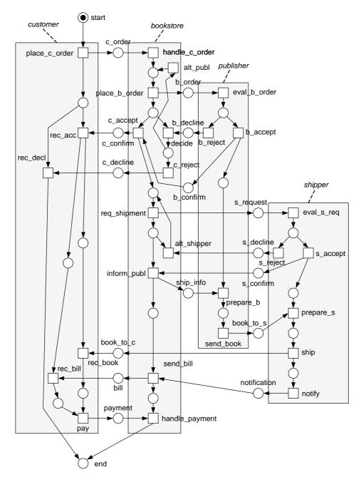
**Fig. 3.** The process as partitioned over (1) the *customer*, (2) the *bookstore*, (3) the *publisher*, and (4) the *shipper*.
