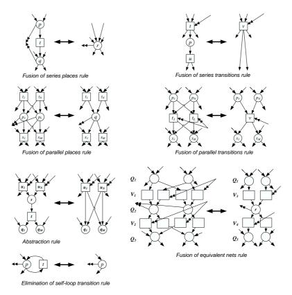
**Fig. 8.** Reset Reduction rules (Please note that the figure does not capture all the requirements for some rules (i.e., if a transition cannot have a reset arc (double-headed arc) or a place cannot be reset, the figure will not show this.)
