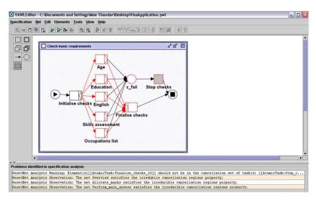
**Fig. 6.** Screenshot of the irreducible cancellation regions property check for modified *Check basic requirements* net
