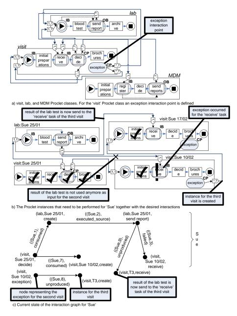
**Fig. 18.** An exception interaction point may be defined for a Proclet class (Figure a). As for "Sue" an exception occurred for the "visit:Sue 10/02" Proclet instance, the exception interaction point has been used for creating a next instance of the "visit" Proclet class which represent the third visit (Figures b and c). Also, the result of the "send report" task is used as input for the third visit.
