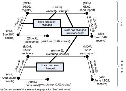
Fig. 13. The "register" task of the multidisciplinary meeting is performed. As performatives have been sent earlier which contain either "(Sue,4)" or "(Anne,4)" as interaction identifier, the task may be completed. Subsequently, the interaction graphs for both are updated.
