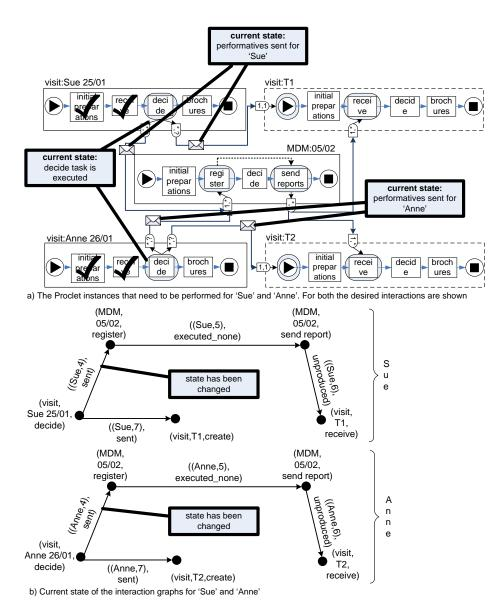
Fig. 11. As a result of executing the "decide" task for both "Sue" and "Anne" in total four performatives are sent. As a consequence, both interaction graphs are updated.
