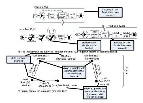
Fig. 6. As a result of receiving the two performatives, instances for the "lab" and "visit" Proclet classes are created. As a consequence, the interaction graph is updated.
