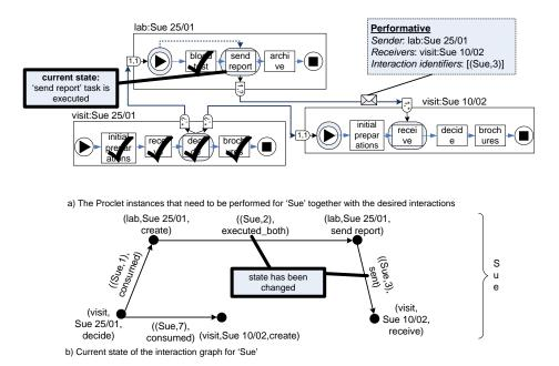
**Fig. 7.** The "send report" task of the "lab" Proclet instance is executed. This results into a performative that is send to the "receive" task of the "visit" Proclet instance for the second visit. As a consequence, the interaction graph is updated.
