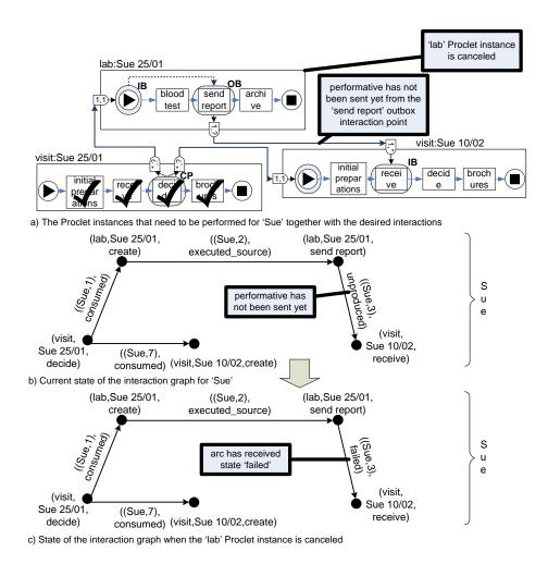
Fig. 20. Illustration of an exception that may occur if a certain Proclet instance is canceled. For a task instance which relates to an outbox interaction point, the required performative has not been sent.
