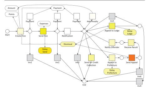
**Fig. 7** Output of the *Projection on net* feature of ProM using a set of balanced alignments. The darker the color, the higher the percentage of deviations that are detected for the transition or the variable. Figure was redrawn to improve readability (ProM does not provide vector graphics)
