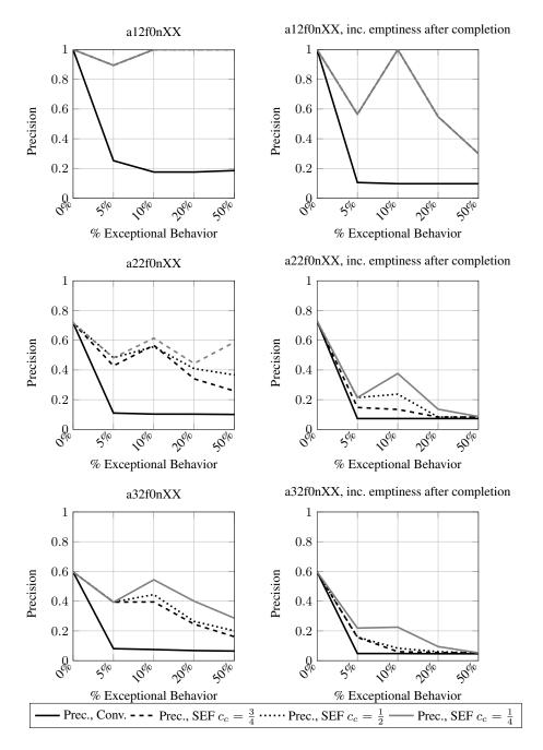
Fig. 11: Precision (Prec.) measurements based on the *a12f0nXX*, *a22f0nXX* and *a32f0nXX* logs. Process discovery based on the conventional ILP-based process discovery algorithm (Conv.) and sequence encoding filtering (SEF) with three different cut-off coefficient values  $\frac{1}{4}$ ,  $\frac{1}{2}$  and  $\frac{3}{4}$ .
