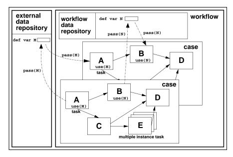
Figure 12: Data interaction between workflow cases
