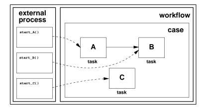
Figure 22: Event-based task trigger
