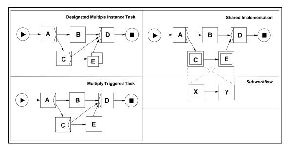
Figure 5: Alternative implementations of multiple instance tasks
