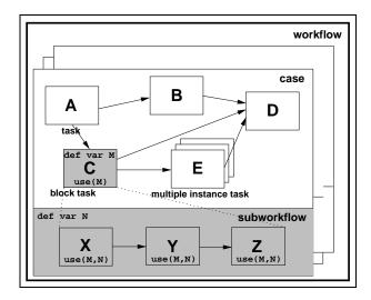
Figure 3: Block level data visibility
